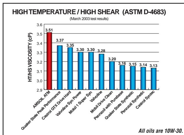
The High Temperature/High Shear Test measures a lubricant's viscosity under severe high temperature and shear conditions that resemble highly-loaded journal bearings in fired internal combustion engines. In order to prevent bearing wear, it is important for a lubricant to maintain its protective viscosity under severe operating conditions.
