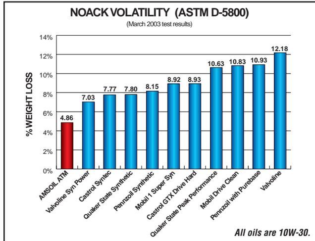
The NOACK Volatility Test determines the evaporation loss of lubricants in high temperature service. The more motor oils vaporize, the thicker and heavier they become, contributing to poor circulation, reduced fuel economy and increased oil consumption, wear and emissions.
