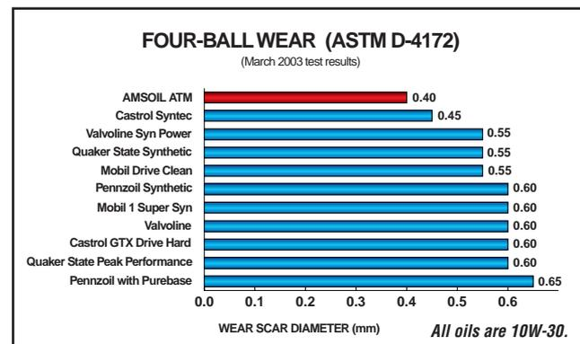
The Four Ball Wear Test determines the wear protection properties of a lubricant. The smaller the average wear scar, the better the wear protection provided by the lubricant.
